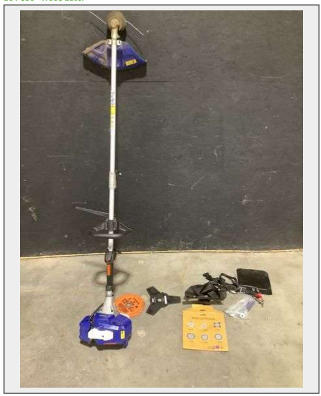
**Description**2 Cycle Trimmer and Brush Cutter. Air Cooled. Straight Shaft 50:1 Fuel/Oil Ratio. Comes with Brush Cutting Blades and Strap.
